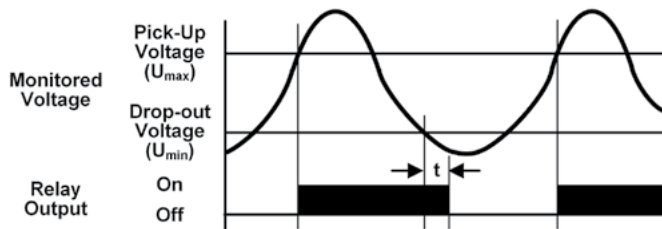
Adjustable Pick-Up, Fixed Drop-Out Settings* Fixed Time Delay on Drop-out at 0.5 Seconds
